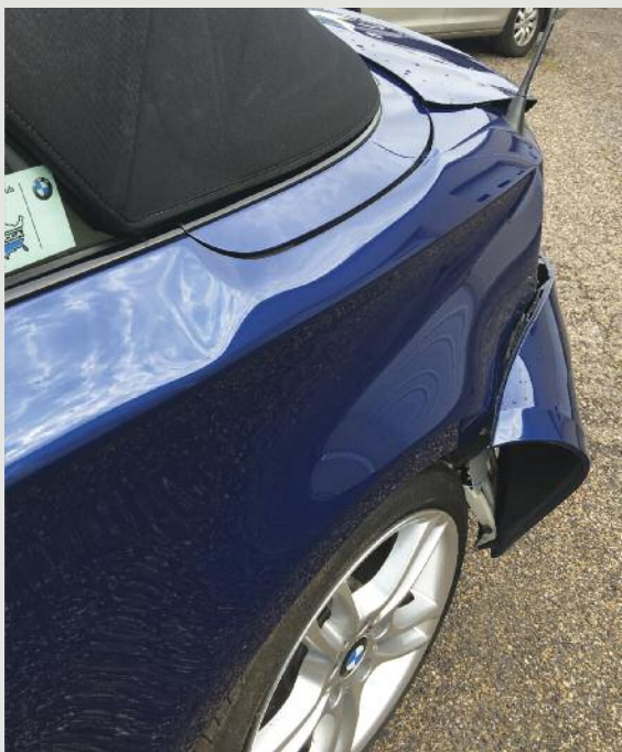
(Below Left) Rear crumple zone worked. (Below Right) Another look at the rear crumple zone.
