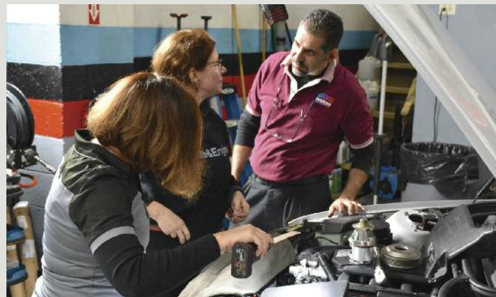
(Top) Bimmer Werks provided a spacious, clean, and organized facility for this NCC DIY. (Above) Amr, Michele, and Jan replace the water pump on the 2002 325xi.
