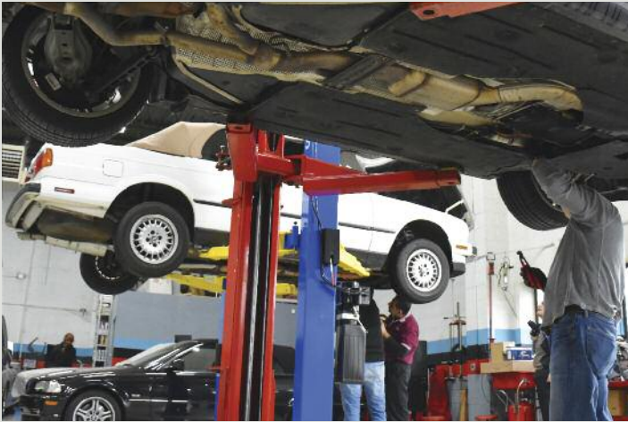
(Above) Brian Montgomery changes the fuel filter on his 2011 535d.
