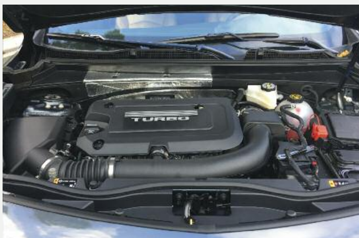
(Above) The XT4 shares the Chevrolet Malibu chassis and transverse mounted drivetrain design.
