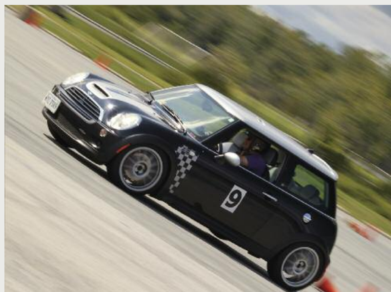
(Below) Wheel Up: Taking the tight corner causes the weight shifting and rear wheel lifting.
