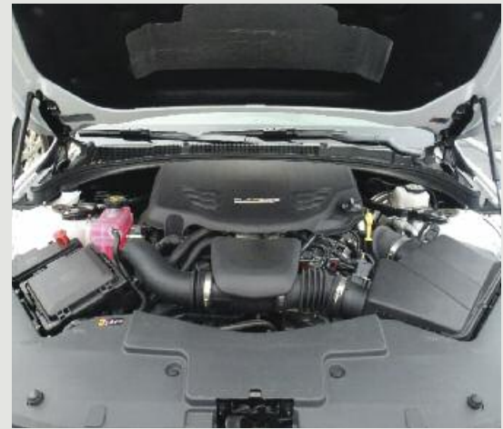
(Above) The ATS-V features a 464 HP, 440 ft-lb of torque, twin-turbo V-6.
