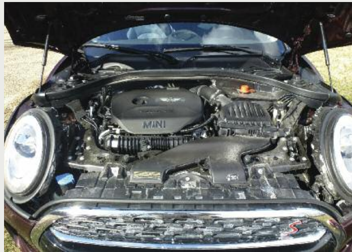
(Above) Along with sharing chassis, the Mini Clubman shares the same modular four-cylinder engine as the BMW X1.
