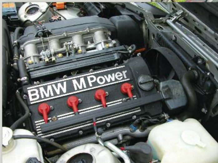
(Top) The E30 M3 in Sterling Silver. (Above) The S14 engine, prototyped in only 14 days, dominated European stock racing for five years.
