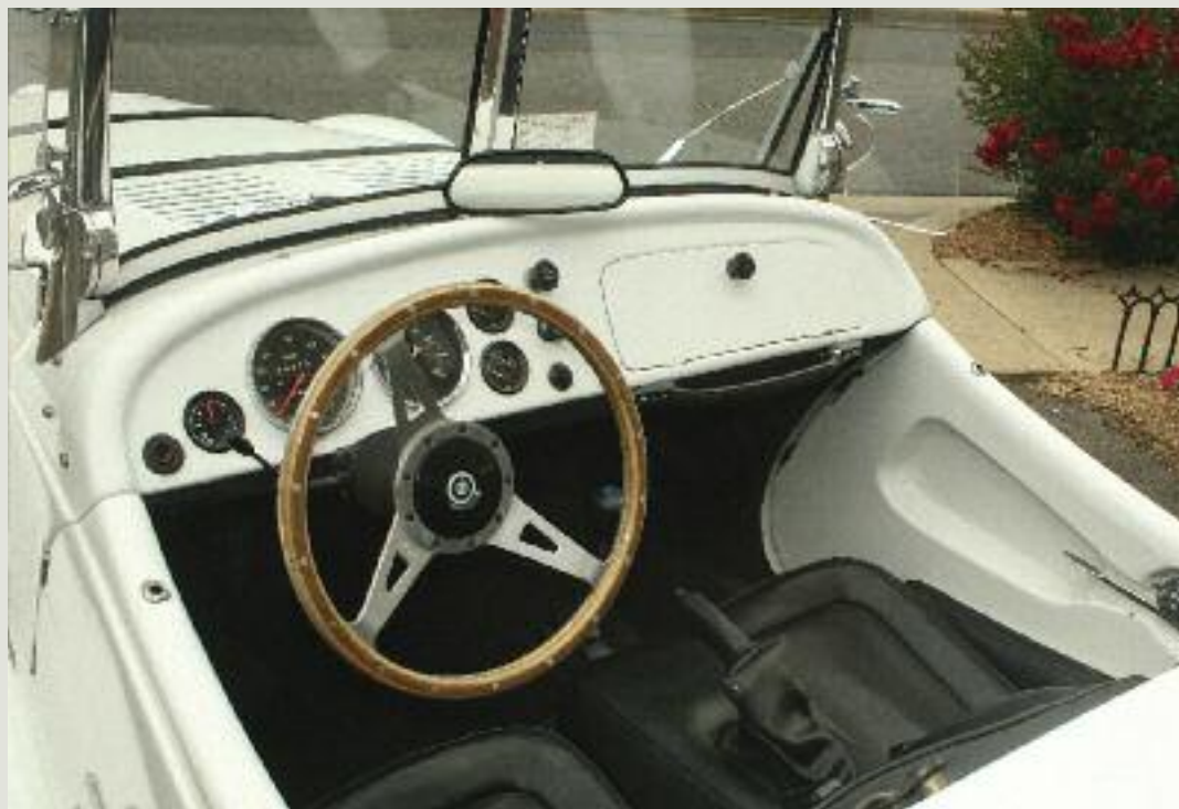
(Above) Frank Sbarro, an Italian native, manufactures replicas of cars of distinction in Switzerland. (Left) Interior gauges are set into the molded dash. The somewhat period steering wheel is large enough to maneuver the NSU front rack.
