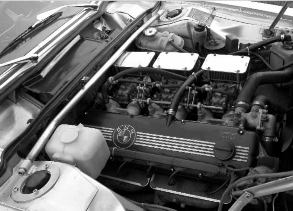
(Top) Three double-barrel Weber 45 DCOE carbs with chrome-plated velocity stacks make a loud and clear statement by this engine. (Below) As an avid autocrosser, Todd bends the old Coupe around the cones with style and perfection. (Right) Early fender treatments are still a trademark of BMW Power.
