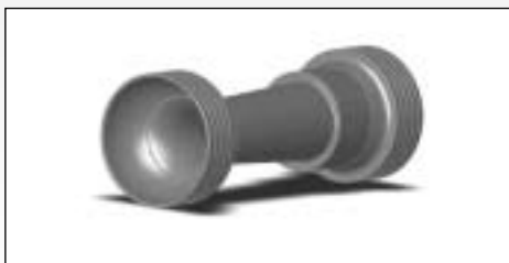
The SCCA-imposed air intake restrictor of 57mm – down from the stock 65mm throttle body opening.
