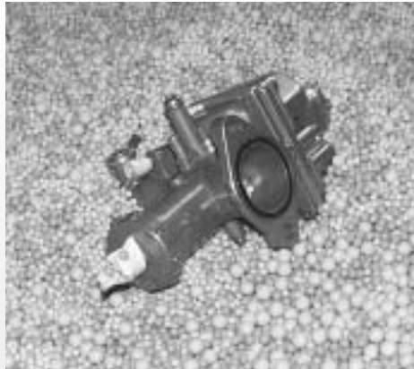
A motorcycle carburetor in the vibratory mill polisher (left). Jeff showing different blast media (lower left). Club members listening intently (below).
