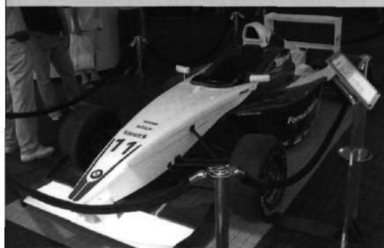
The Formula BMW USA series car is powered by the 1.2-liter engine from BMW's K 1200 RS motorcycle. The inline-4 makes 140 bhp and 86 lb.-ft. of torque. Photo: Raine Mantysalo
