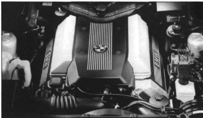
BMW 4.0 Liter V-8...The all-new liter V-8 engine is standard equipment in the BMW 740i and 740iL. Features include aluminum alloy block and cylinder heads, dual overhead camshafts, 4 valves per cylinder and the latest generation of BMW's Digital Motor Electronics engine management system. Designed for low maintenance, the 282 horsepower V-8 is coupled to an electronically-controlled 5-speed automatic transmission with three shifting programs.
