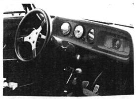
This is the cockpit of a CSL. Note complete VDO gauges (as can be found in any Porsche 911S), and position of tachometer (that's right, a 9,000 redline).
