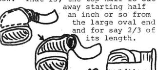
Vents are now installed in the shelf but open into the trunk. The air now passes into the trunk itself and through the large cutout in the pipe and out under the lip. Thus, the air vents through the trunk rather than down flex hoses. By leaving the bottom half of the pipe in place, any water that works its way into the pipe remains trapped in it and not in the trunk.
