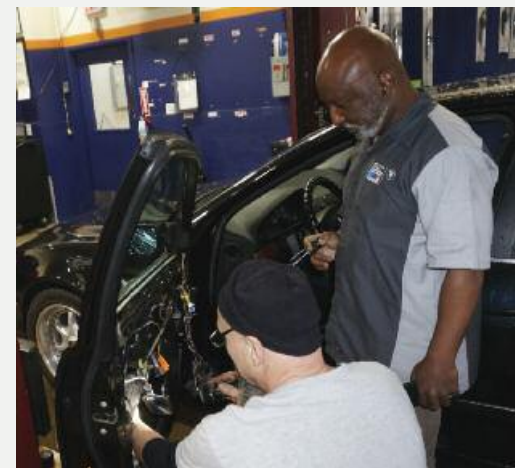
(Below from Left) Joseph Concaugh removes the DISA valve on his E46 to gain access to clean the throttle body and ICV; Jedd Vertman removes a wheel from his 2004 325xi to begin replacing his brakes and rotors; Mike Reynolds from Craftsman Auto Care helps Phillip Cummings replace the window regulator on his E39 540i.
