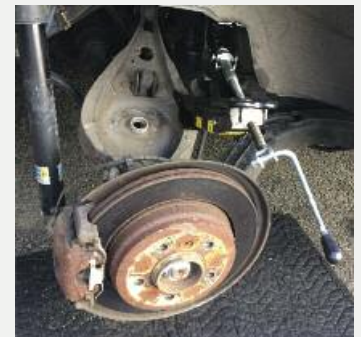
(Middle from Left) The author's broken rear coil spring next to a new replacement; after you remove the lower bolt holding the rear shock in place, you can use a scissor jack to gain enough space to remove the coil spring.
