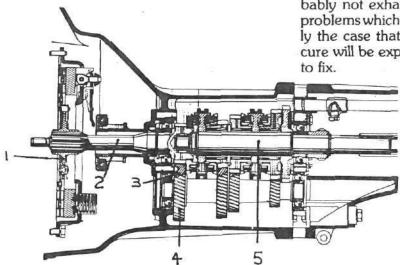
the layshaft is in motion. The layshaft perman ently turns gears on the output shaft (5), which looks like it is attached to the input shaft but in fact is not — it is separated by a bearing, and is coupled to the input shaft only when fourth gear is selected. So, in neutral position clutch engaged, the input shaft, layshaft and output shaft gears are all spinning. How does one select a gear? Moving the gearshift lever causes a shaft to move a fork, which pushes a ring over
